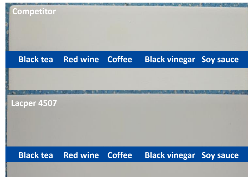
Stain resistance test (1h)
