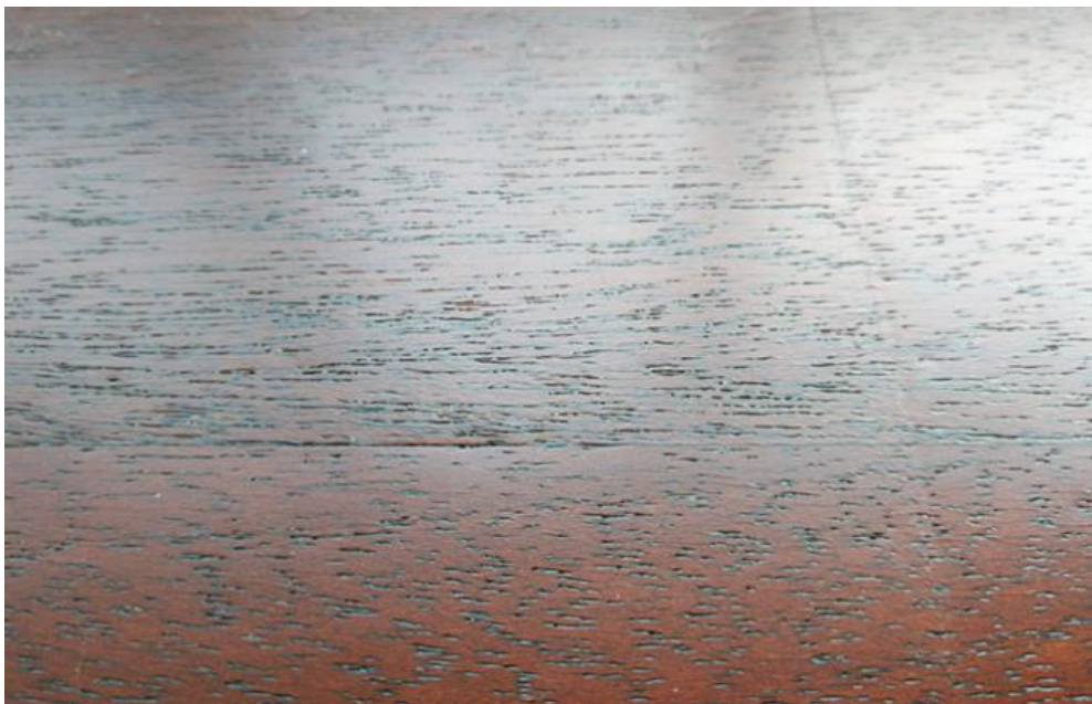
Lacper® 4101 on mahogany substrate Excellent penetration without 'crater'
